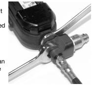
new jam nut against the Quick Fill Adapter Block and torque to 200 - 225in.lbs with a thin crowsfoot wrench.
