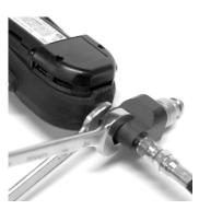
3. Unthread ICM unit from Quick Fill Adapter Block.
